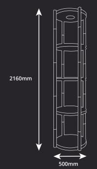
Depth: 500mm Weight: 20kg Internal Shelf Load Bearing: 4kg Internal Shelf Height: 500mm Internal Shelf Size: 460mm Dia
