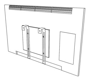
Mount the TV by guiding the hooks through the cut holes and securing them onto the top crossbar. The TV hooks will rest on the bottom bar, ensuring the TV does not ripple your graphics.
