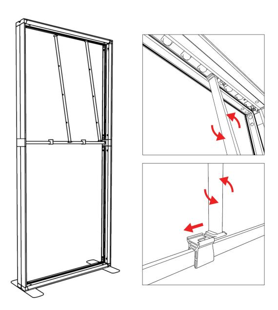
Attach the horizontal metal bars using screws, with the bar positioned at the front of the lightbox and screws at the rear. The wider metal bar should be placed at the bottom to provide support for the TV.
